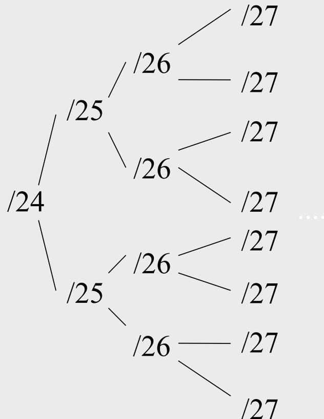
By adding one bit to the netmask, we subdivide the network into two smaller networks. This is *subnetting*.
