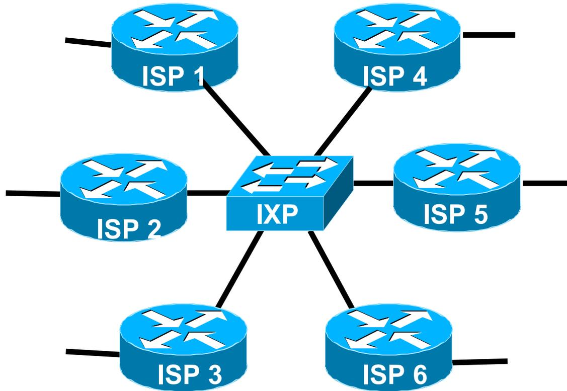
**Each of these represents a border router in a different autonomous system**
