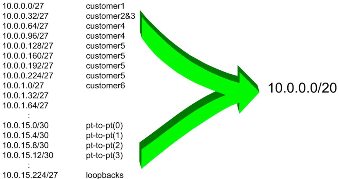
Figure 3 – Extract from an ISP addressing plan
